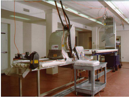
Figure 3. Primary processing line showing airdraft cleaner and washing/drying unit.
