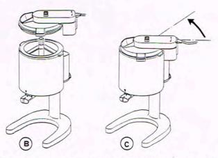
6 Plug power cord into 120 Volt AC outlet. Turn switch on. Note: The ice cream container stays still while dasher rotates inside it.
