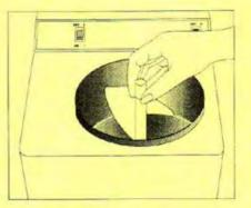
\*REMINDER: Always be certain the mixing bowl and interior copper lining are COMPLETELY DRY before using the "chill". This will prevent the bowl from "icing up" and interfering with the cooling process.
