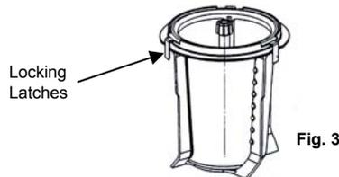
4. Place the canister assembly into the slushie container, ensuring that the ice canister sits flush onto the drive spline at the base of the slushie container.
