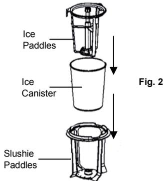
3. The locking latches on the ice paddles should easily snap onto the slushie paddles. (Fig. 3)
